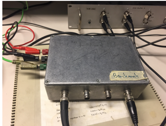
Figure 5.1 – Picture of the Wiener-Hammerstein system.
